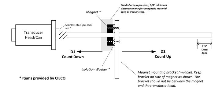
Use the 3.4" (19 mm), 16 UNF thread of the transducer to mount it at the selected location. Install the permanent magnet over the LDT rod. Mount the permanent magnet to the movable device whose displacement will be measured.
